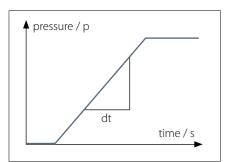
For SUCO electronic pressure monitoring products the maximum pressure change rate can be up to 5 bar/ms (5,000 bar/s).
