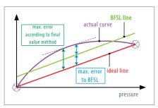
Non-linearity is also shown as BFSL (Best Fit Straight Line) as a reference value in the technical specifications. Non-linearity generally has the biggest influence on the overall error rate. Typically, non-linearity as per BFSL corresponds to half of non-linearity as per the full scale method (1% FS  $\sim$  0.5% BFSL).
